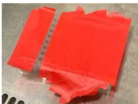
Figure 2. Moving lab tape on the SSP to expose one column at a time.
