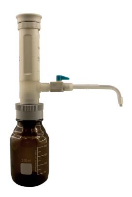
Corrosive substances may damage the adapter Check the chemical resistance befor using organic solvents or aggressive chemicals.
